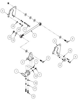
NOTE: There are two (2) axle brackets in this kit. One fits the 110/115 rear axle and one fits the 135/150 rear axle. Match the bracket to the bolt pattern and discard the bracket that does not fit.
