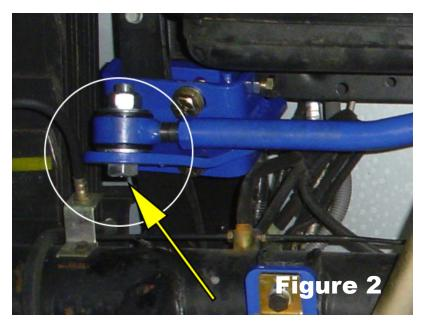
Frame Bracket Bolt Must Be Inserted As Seen Above To Prevent Damage To Brake Line Attached To Axle.
