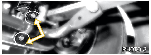
Remove two bolts from one side (PHOTO 3) and install the SS403-3 axle bracket with the round end upwards and angle towards the rear.
