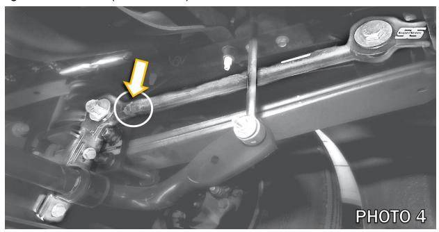
Adjust the radius rods to length and install from axle bracket to frame bracket with  $\frac{3}{4}$ " x 3" bolts, flat washers and lock nuts capturing the bushings on both sides with the flat washers.
