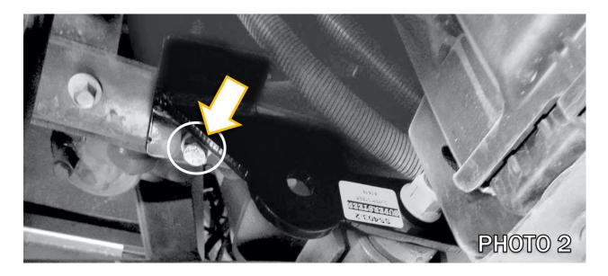
Align the hole in the bracket with the hole in the frame and install the new  $\frac{1}{2}$ " x 1.5" bolt with flat washer from the bottom up (**PHOTO 2**) through the bracket and frame with flat washer and nut on top side.
