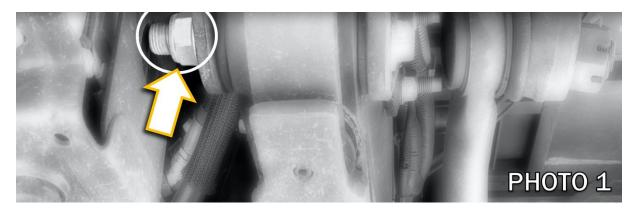
Remove the nut (PHOTO 1) from the forward spring eye bolt (15/16 wrench for nut)(13/16 or 21mm for bolt head)
