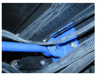
Begin by removing three nuts and bolts from the joust bumper (on the driver side of the frame) as needed to bolt on **frame bracket**. Install the **frame bracket** on the inside of the frame by using the supplied bolts, nuts and washers. Torque to 100 ft. lbs.
