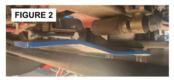
Place Brass Plunger (Item 8) on push rod of Air Chamber (Item 7) and install on Sleeve/Bolt Assembly (Item 6) using two 7/16" Coarse Lock Nut and Washer (Item 28). Make sure that the brass plunger aligns with machined slot on bolt slide area.
