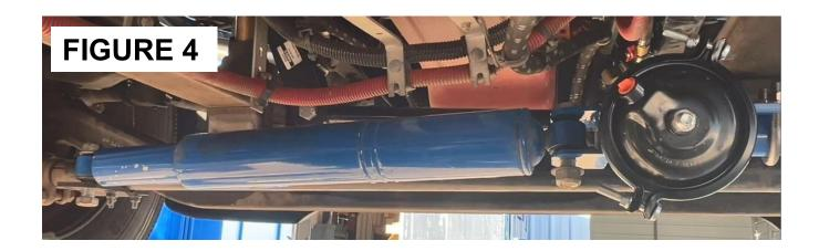
Important: With Cylinder installed, again check to confirm there is sufficient clearance around all moving parts with steering turned from lock to lock, accounting for suspension travel, with coach at ride height. If Cylinder scrapes or binds at any point, review instructions and make necessary corrections by rotating Tie Rod Bracket and/or Sleeve/Bolt Assembly to obtain necessary clearance.
